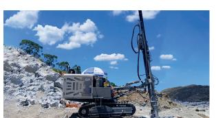
**Mobility / Stability:** Designed with hydraulic planetary reducers, making it self-sufficient for movement, delivering high torque and excellent uphill performance.
