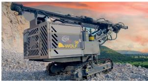
Lowest Diesel Consumption in its Category: Diesel consumption of 13 to 15 liters per hour, depending on drilling diameter, rock type, and conditions, along with reduced pollutant emissions (compliant with TIER 3 standards).
